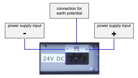
Figure 11: DC voltage connection at power supply
