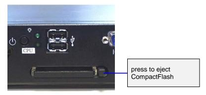
Figure 8: CompactFlash adapter
